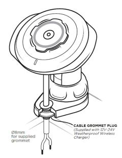
2. CABLE PASS THRU GROMMET PLUG UNDER COVER
